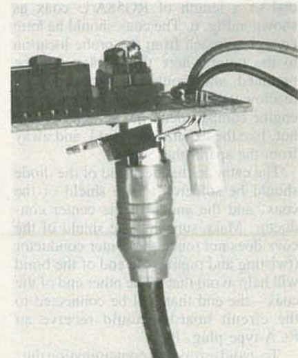
FIG. 4—BEND IC1 OVER BACKWARD on the bottom of the board as shown.
