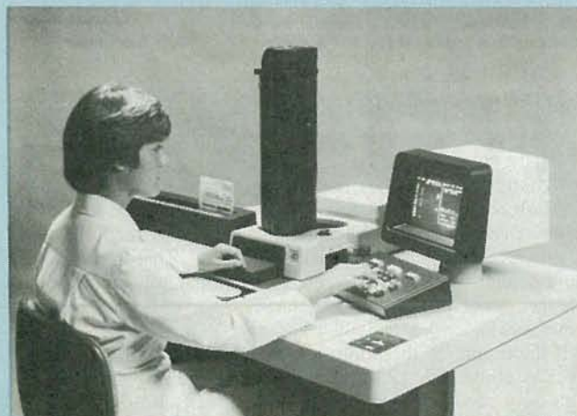
FIG. 6—THIS CONSOLE lets the operator encode information in the disc's magnetic core. That information can be read automatically by special printers.
