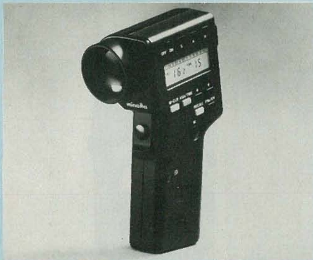
FIG. 5—THE SPOTMETER is a special type of reflected-light meter. Shown is the Spotmeter M from Minolta.
