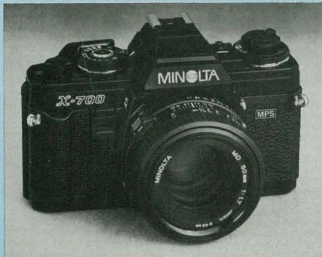
FIG. 1—THE MINOLTA X700 represents the ultimate in autoexposure technology and flexibility. It features a program mode in which both the aperture and the shutter speed are determined by the camera, an aperture-priority automatic mode, and a fully metered manual mode.
